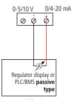
Connection of output in voltage 0-10 V:
